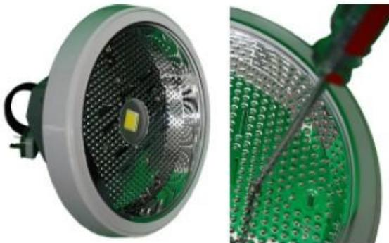
**Step 4: Insert the clip into the socket at the reflector.**
